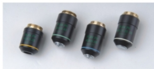
PLAN-PH series infinity phase contrast objectives. In addition to the realization of the bright field observation, the phase contrast observation function has been developed. they especially suit colorless or undertone cells.
